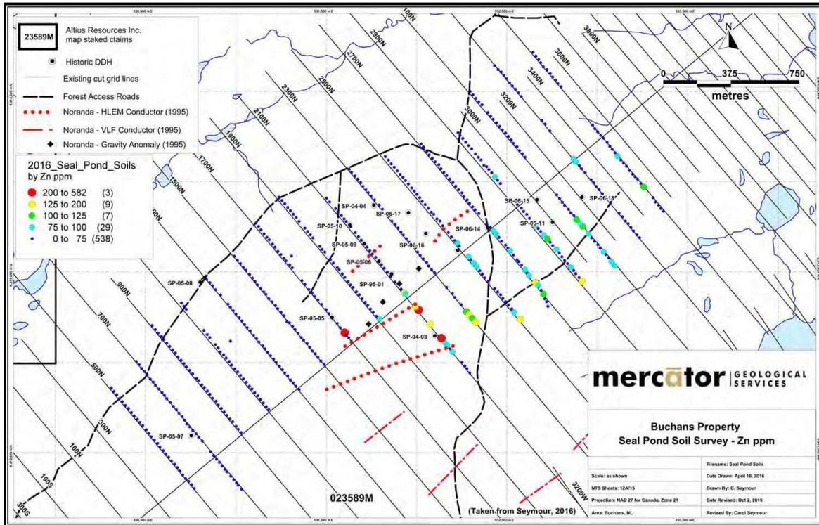
Previous work in this soil grid area by Noranda identified northeast trending electromagnetic (EM) survey conductors with coincident IP chargeability anomalies. In 1970, Asarco drilled two holes in this area (H2817 and H2819) and H2817 intercepted 0.71% Cu over 1.5 m.
