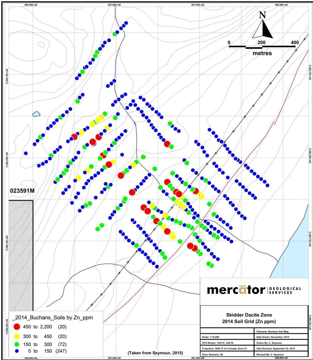
Figure 9.2: Skidder Dacite Area soil survey zinc (Zn) results
