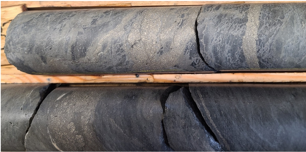
Photo 3. Sulphide stringers and disseminations in altered rhyolite drill core at approximately 433 metres down-hole in MM-26-41 1 .
