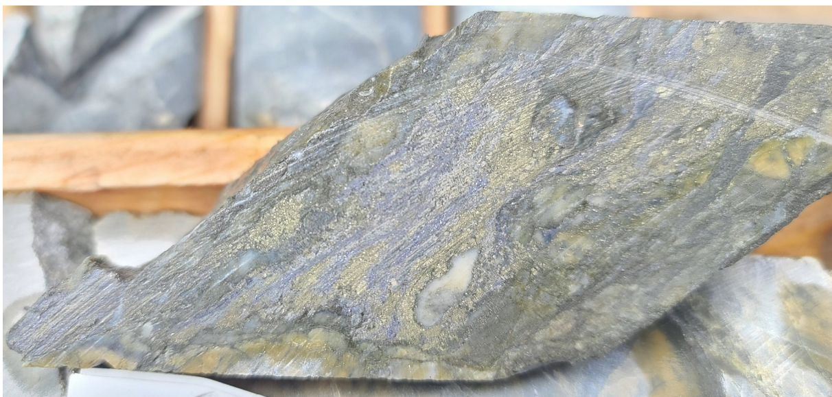
Photo 2. Cut core face at approximately 417 metres down-hole in MM-26-41: banded pyrite stringers with grey sphalerite in strongly altered rhyolite 1 .
