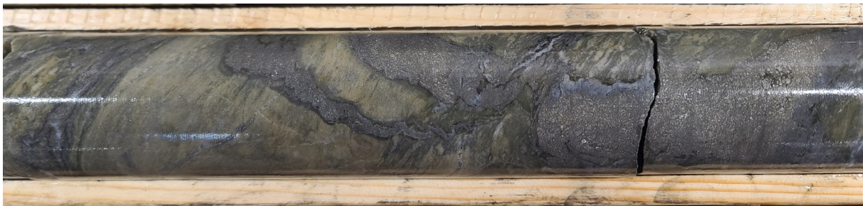
Photo 1. Pyrite stringer mineralization in altered rhyolite at approximately 414 metres down-hole in drill hole MM-26-41, within the approximately 118-metre interval of strongest stringer development 1 .
