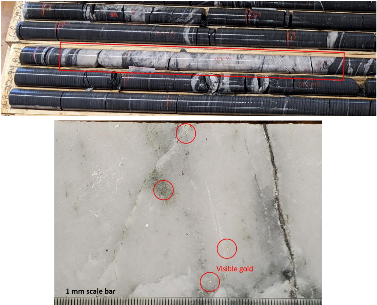
Figure 3 - Drill core from GB-22-94 with large quartz vein starting at downhole depth of 47.8 m (visible gold within red circles)
